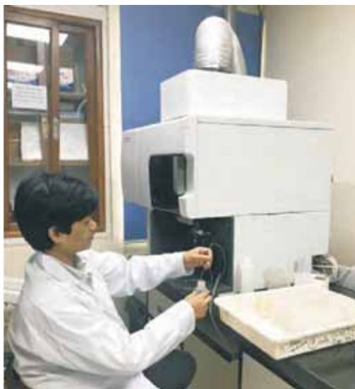
Inductively Coupled Plasma - Optical Emission Spectroscopy (ICAR-Indian Agricultural Research Institute, New Delhi)
